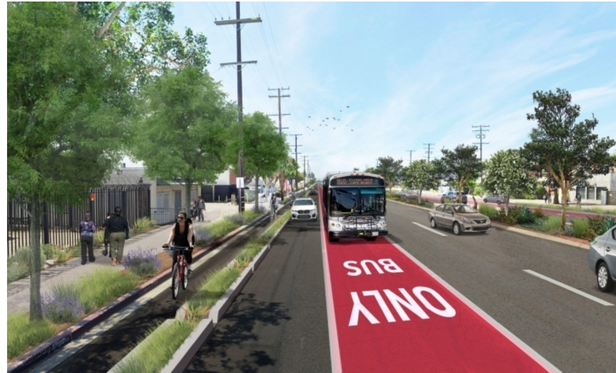
Complete Street with Side Running BRT
